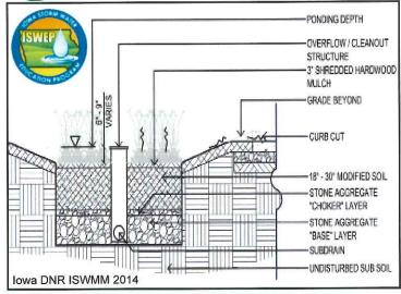
Bioretention cells are engineered to infiltrate, percolate and filter stormwater runoff. Attention must be given during construction to prevent compaction and prevent sediment from clogging the modified soil mix.
